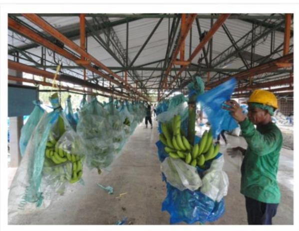
**Cableway carries bananas to the packing plant**
